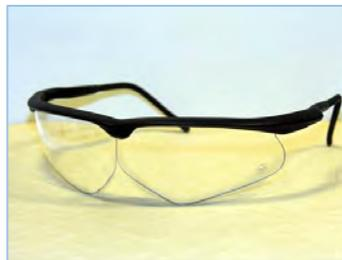
*Safety glasses used for shooting should have a clear, distortion-free area near the bridge of the nose. Target shooters look through this part of the lens when aiming.*
